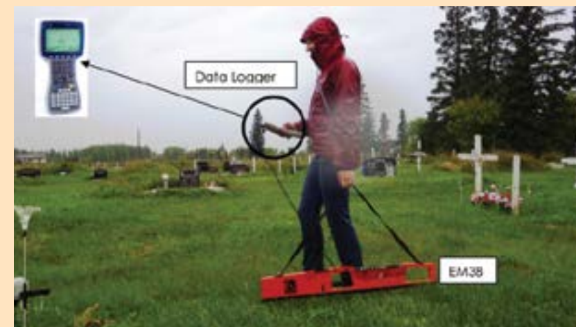
EM38 and Allegro data recorder in operation (© Stantec Consulting Ltd.).
